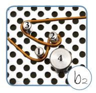
b2- Measure and cut at least 15 cm of wire and roll the wire around starting from peg 1. Make a loop around peg 2 and then go around peg 3.
