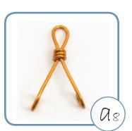
a8-Once the three turns are completed, cut off the excess wire.
