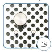
3-Insert 3 pegs (2 small and 1 large) as illustrated on the left. Do not forget to block the pegs behind the Jig with the rubber pieces.
