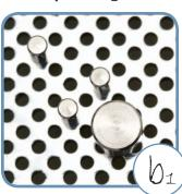
b1-Insert 4 pegs (3 medium and 1 large) as illustrated on the left. Do not forget to block the pegs behind the Jig with the rubber pieces.
