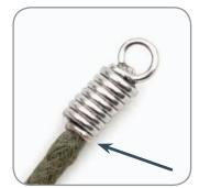
Glue the tip of the cord and insert it in the connector.
