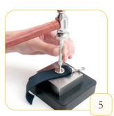
3- Install the female part of the rivet on the male one, the hole that receives the snap facing upwards.
